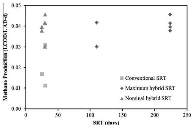
**Fig. 2.** Average methane production by phase from the hybrid and conventional processes as functions of nominal and maximum SRTs. Nominal SRT is calculated from Eq. (1), and maximum SRT is calculated from Eq. (4).
