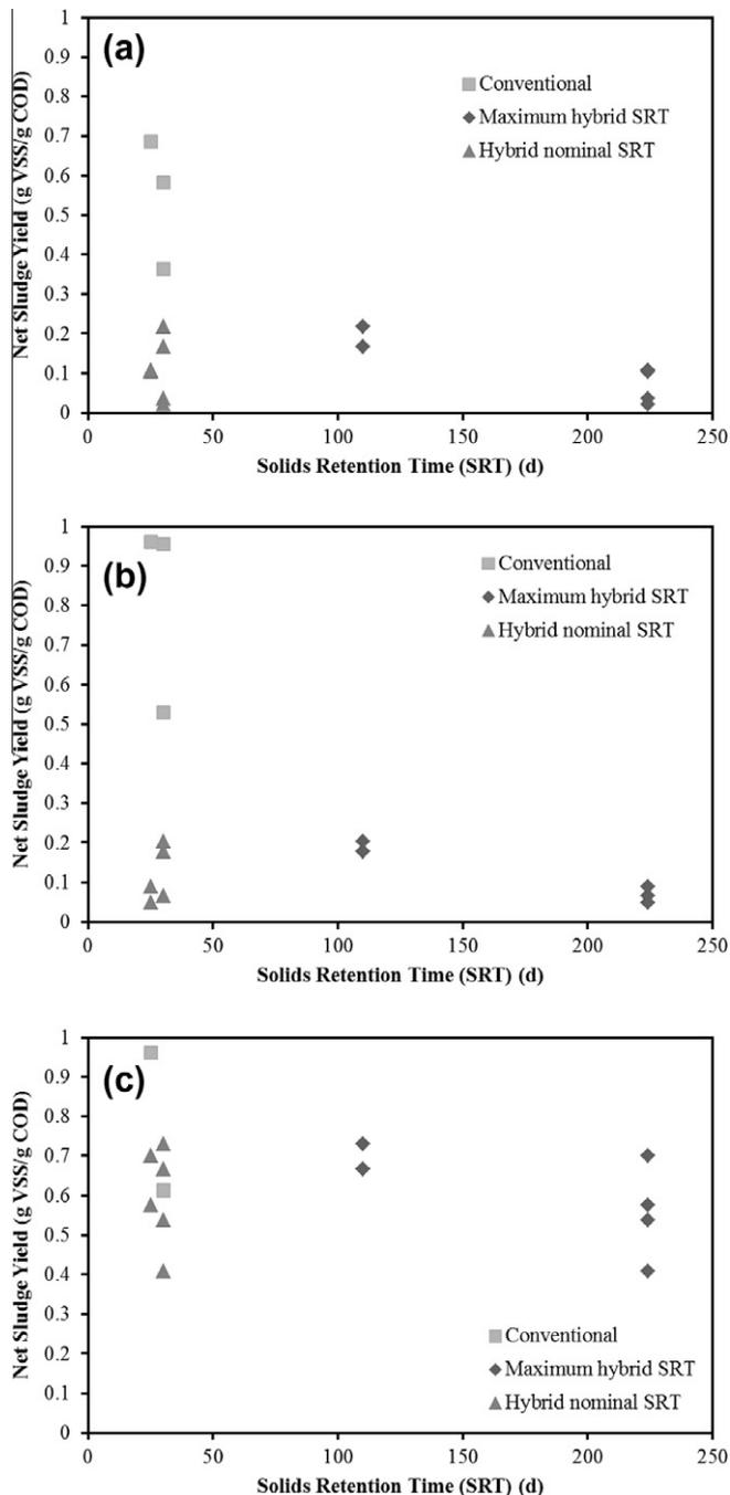
**Fig. 4.** Net average net sludge yields by phase in the hybrid and conventional processes (a) for the total system (Eq. (5)), (b) from the AD using the wasting sludge only, and (c) from the AD taking into account the total flow leaving the AD. SRTs are calculated based on Eq. (1) for nominal SRT and Eq. (4) for maximum SRT.
