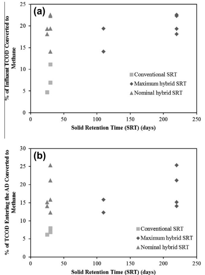
**Fig. 3.** Average percentages of (a) system-influent TCOD and (b) TCOD entering the AD converted to methane by phase in the hybrid and conventional processes as functions of nominal SRT (Eq. (1)) and maximum SRT (Eq. (4)).
