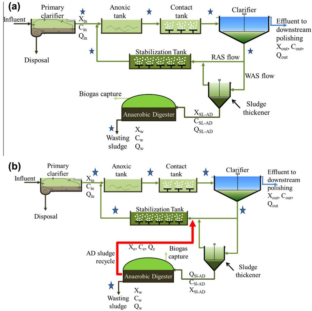
**Fig. 1.** (a) Conventional process with contact stabilization and anaerobic digestion. (b) Hybrid process with contact stabilization, anaerobic digestion, and digester-sludge recycle (heavy line). Variable labels include  $Q$  for volumetric flow rate ( $L^3/t$ ),  $C$  for concentration ( $M/L^3$ ), and  $X$  for biomass concentration ( $M/L^3$ ). Stars represent sampling points for methanogens assay.
