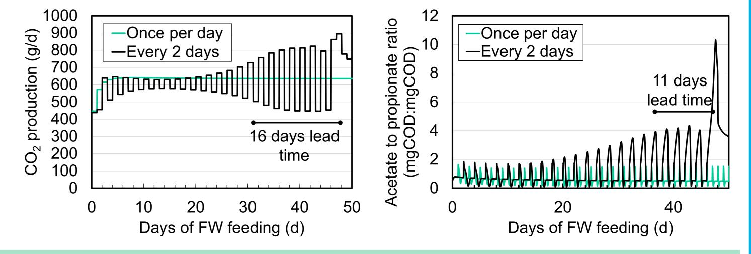
**Leading indicators of souring:**  $HCO_3^-$  was the indicator with the longest lead time. While  $HCO_3^{-1}$  is difficult to quantify directly, it can be determined from the difference between total and VFA alkalinity. Ratios of VFA:SCOD, SCOD concentration, NH4+ concentration, and solids reduction did not indicate souring until pH decreased to < 6.0.
