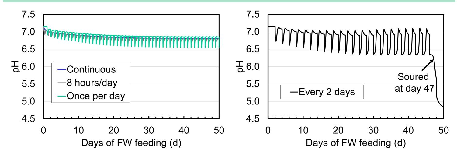
The digester fed every 2-d had longer term decrease in  $HCO_3^-$  alkalinity due to two phenomena related to pH: (1) longer accumulation of VFAs, especially acetate,
