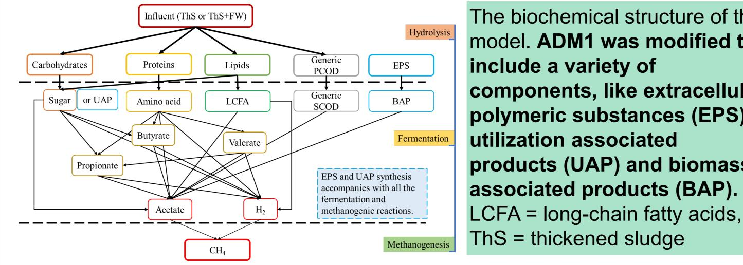
The biochemical structure of the model. ADM1 was modified to include a variety of components, like extracellular polymeric substances (EPS), utilization associated products (UAP) and biomass associated products (BAP).
