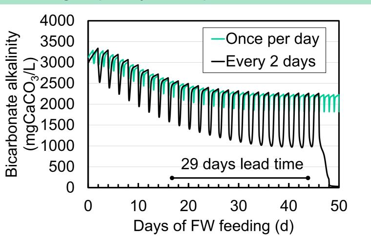
$HCO_3^-$  alkalinity < 1500 mg  $CaCO_3/L$  is often cited as the lower threshold for safe operations of traditional anaerobic digesters<sup>2</sup>. Because the daily  $HCO_3^-$  fluctuates with intermittent feeding, this criteria is less applicable.
